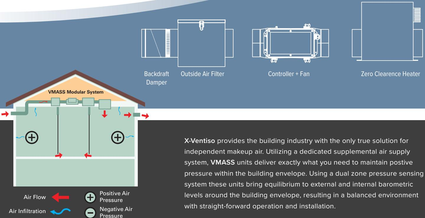
X-Ventiso provides the building industry with the only true solution for independent makeup air. Utilizing a dedicated supplemental air supply system, **VMASS** units deliver exactly what you need to maintain positive pressure within the building envelope. Using a dual zone pressure sensing system these units bring equilibrium to external and internal barometric levels around the building envelope, resulting in a balanced environment with straight-forward operation and installation.
